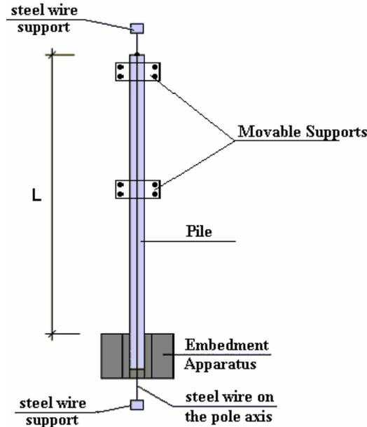
Figure 4 – Hinged movable supports for the pile
